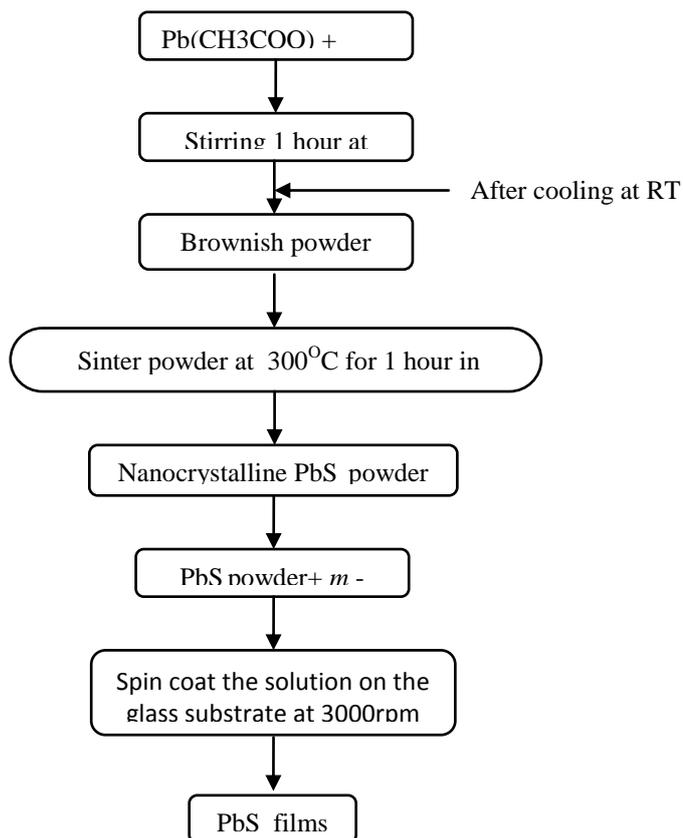
Figure 1. Flow diagram for PbS films prepared from the novel chemical process using the spin-coating method
