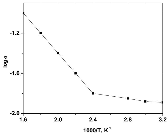
Figure 4 . The temperature dependence of an electrical conductivity of PbS film
