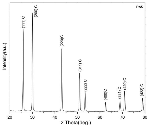
Figure 2. X-ray diffraction of PbS films
