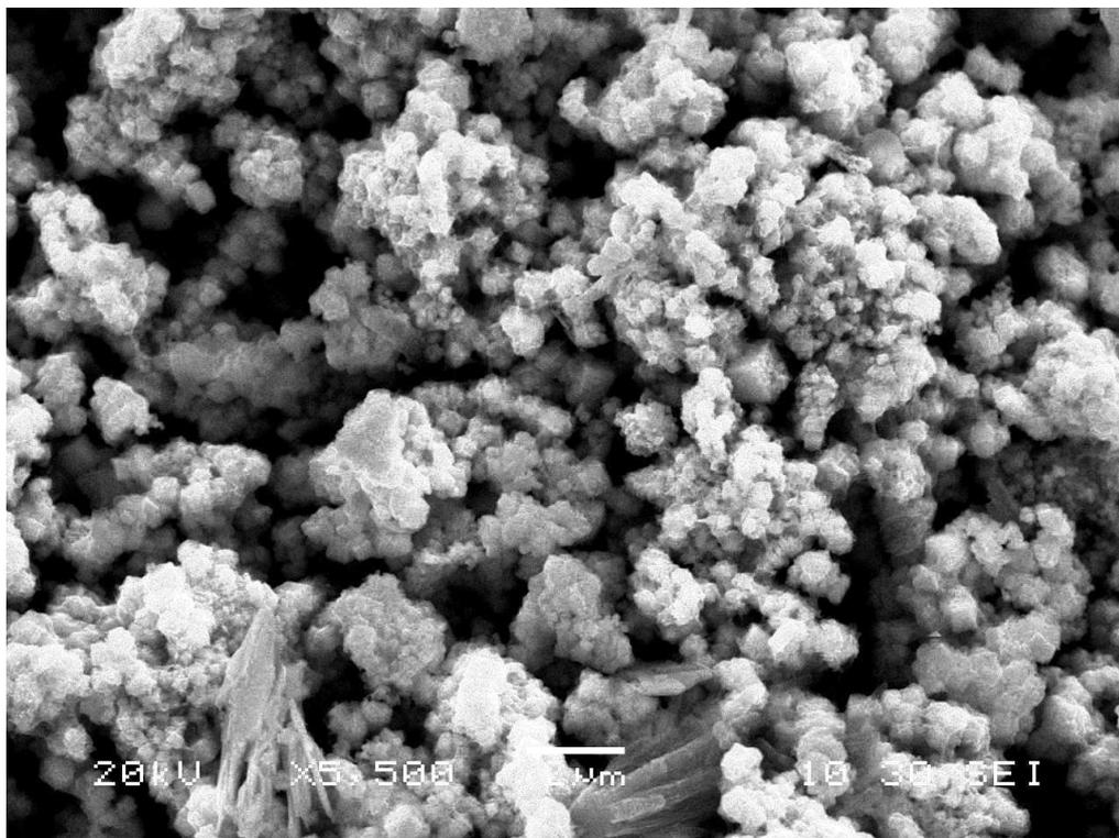
**Figure 3.** shows the SEM image of nanocrystalline PbS films
