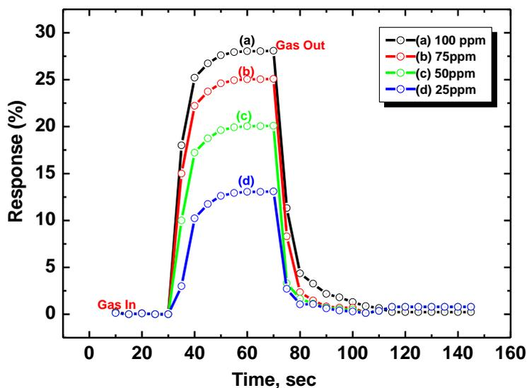
**Figure 7. Dynamic variation of the response of the PbS thin film with time**
