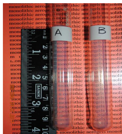
Figure 4: Photograph of monolithic Silica aerogels
